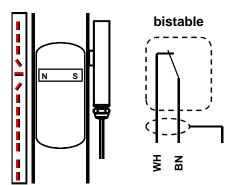
" Installed opposite to indication rail " Cable exit downwards
